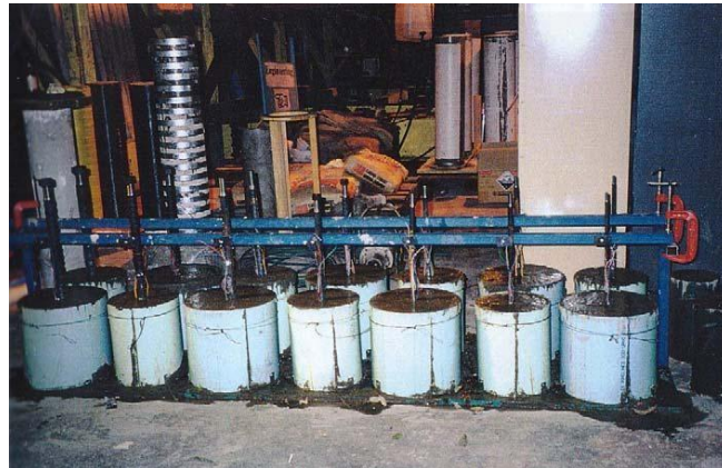
Fig. (4). Casting the specimens.
