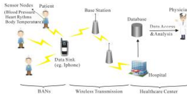
Fig.1. An Basic Architecture of the E-health System
